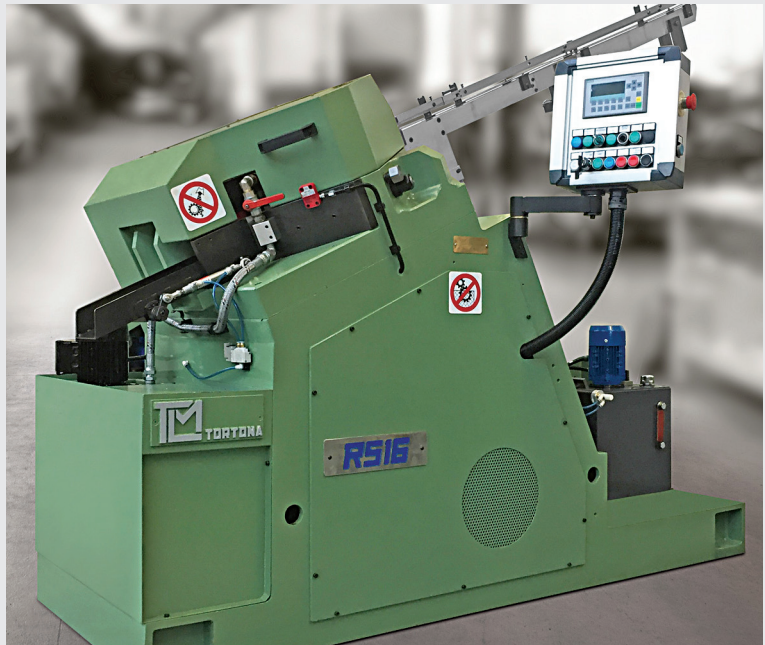
TLM RS16 Thread Rolling Machine
